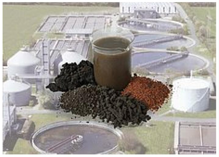
The better wastewater is treated, the more sludge is generated thereby. Primary sludge consists of solids removed from raw wastewater. Secondary sludge consists of biomass generated by biological treatment. Tertiary sludge is generated by advanced chemical/physical treatment.
